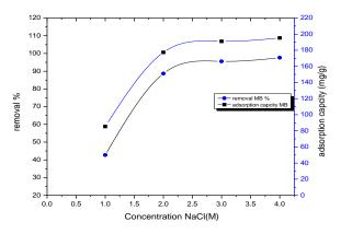
**Figure 6.** Effect of salt addition on the adsorption processes of BALS and MB (rpm: 300; pH: 5.90at MB at Temperature room at C0 100 mg/l
