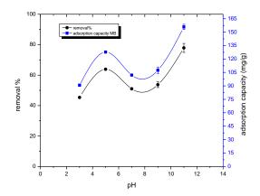
**Figure 3.** Effect of pH on the removal percentage andadsorption capacity under condition Co 100 mg/L, 300rpm, 120 min, dosag 0.01g, 20ml, room temperature
