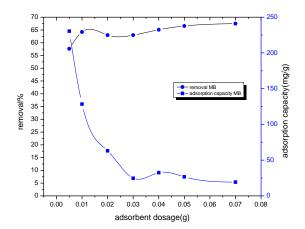
Figure 1. Effect of adsorbent dosages on the removal and adsorption capacity of BASS under
