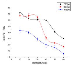
**Figure 1**. Effect of temperature on removal percentage the adsorption processes of BALS and MB under condition Co 100mg/g, dosage 0.01 g, 20ml, pH=5.90, 300rpm, 120min
