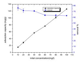
**Figure 4.** of initial concentration on removal and adsorption efficiency under condition dosage 0.01 g, 20ml, pH=5.90, 300 rpm, 120min, room temperature
