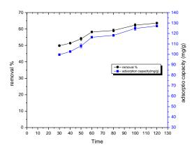
**Figure 2.** Effect of time contact time on the removal and adsorption capaity under conditions Co 100 mg/L, 300 rpm, dosag0,01g, 20ml, pH=5.90, roon temperature.
