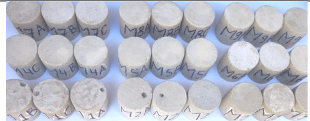
Fig. 9: The Prepared Hardened Cement Mortar Samples with Various (SLS %).
