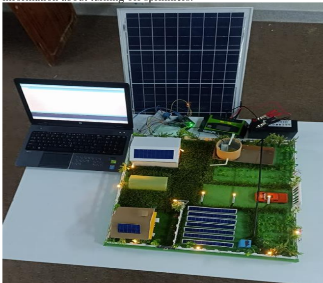
Fig 4. A solar panel is used for battery charging
