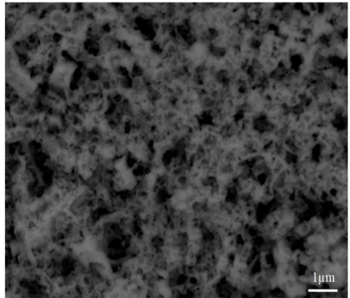
**Fig. 3** Scanning electron microscope (SEM) micrograph of the MOF-5 and Mesh.
