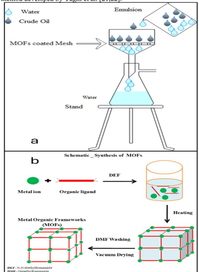
**Fig. 1.** (a) Schematic diagram of the separation process using the MOFs coated mesh (two-stage process mesh and polish). (b) Schematic diagram of the synthesis of the Metal-organic framework (MOFs).
