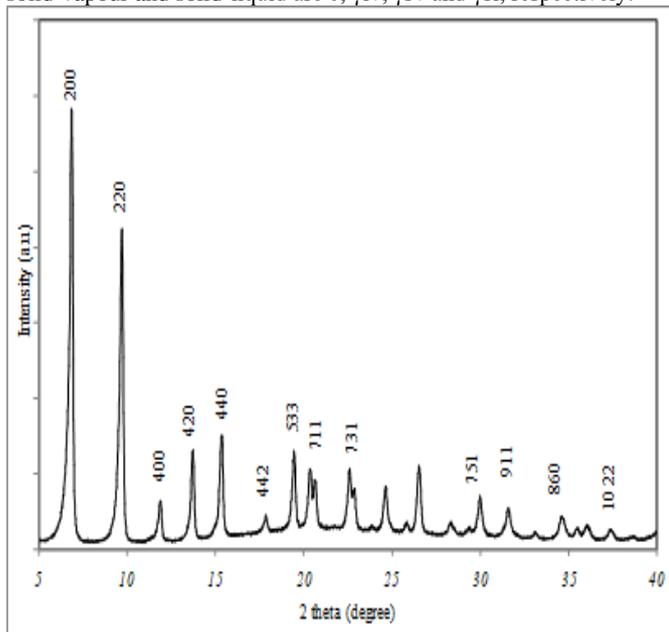
**Fig. 2.** X-ray diffraction pattern of the MOF-5
