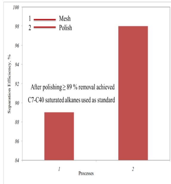
**Fig. 6** Separation efficiency for two processes of MOF-5/PDDA coating.
