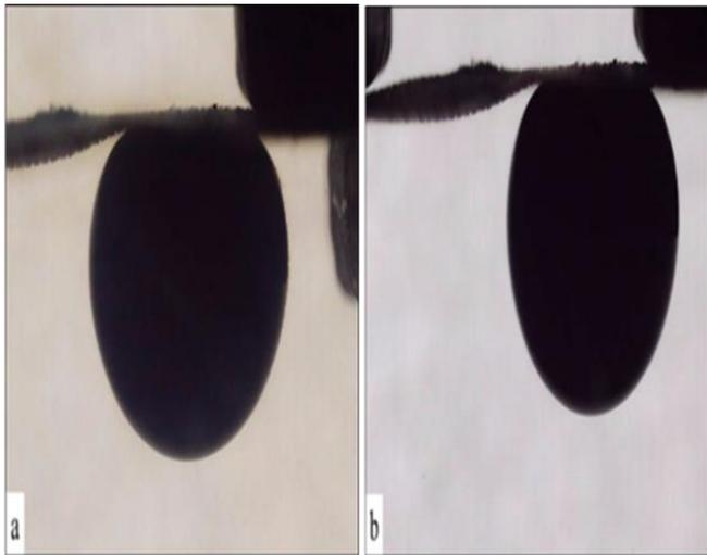
**Fig. 5** (a) Contact angle of the crude oil on the mesh coated with MOFs, (b) Contact angle of the crude oil on the mesh coated with MOFs/PDDA.
