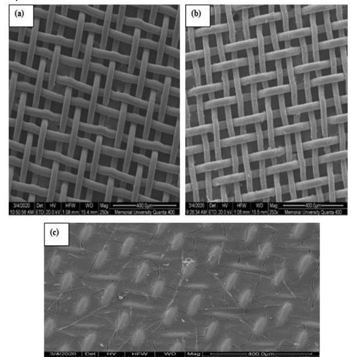
**Fig. 4** (a) SEM image of the mesh, (b) SEM image of the mesh coated with MOF-5, and (c) SEM image of the mesh coated with MOF-5 and PDDA.
