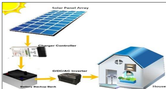
Fig. 1. Shows the components of the solar energy system.
