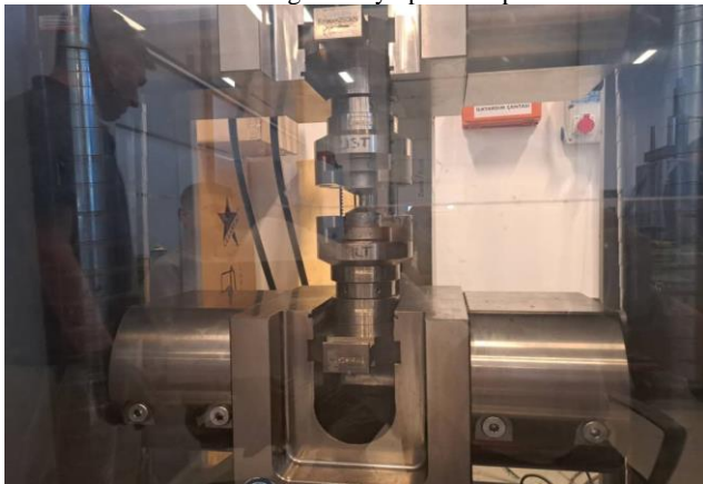
Figure (3) : Tensile testing machine with an extension parts to test short samples.
