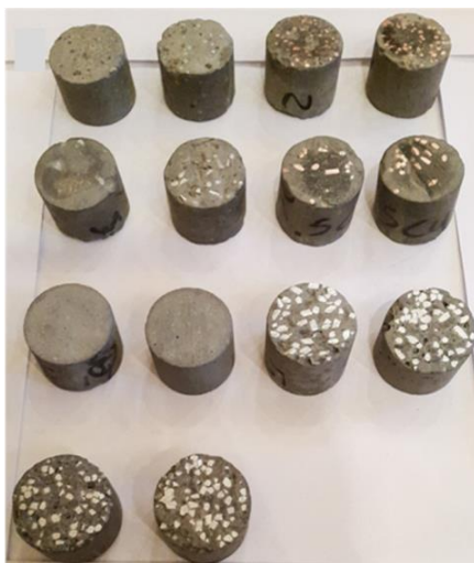
Figure 2.8 –The types of samples following the process of cutting, surface finish and weight measurement
