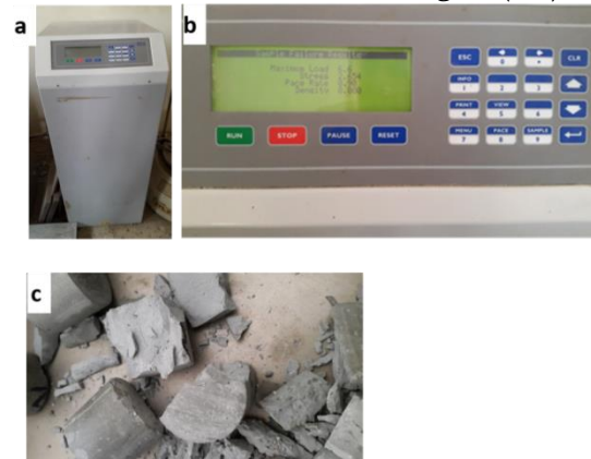
Figure 2.9 – a) and b) ELE international compression machine, c) showing sample after crushing test.
