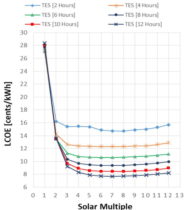
Fig.7: Levelized Cost of Energy for 100 MW Parabolic Trough Plant
