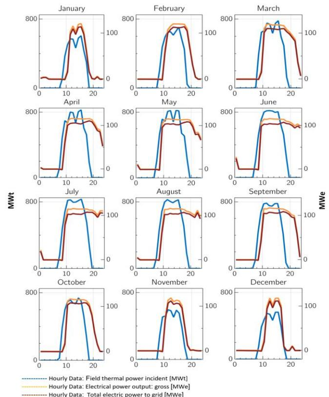
**Fig.4:** Hourly data of field thermal power incident, gross electrical power output, and total electrical power to grid for the proposed plant in Sebha.
