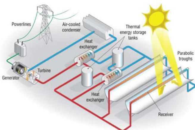
Fig.1: System Advisor Model (SAM) sketch of a parabolic trough plant. Credit NREL/SAM [19].
