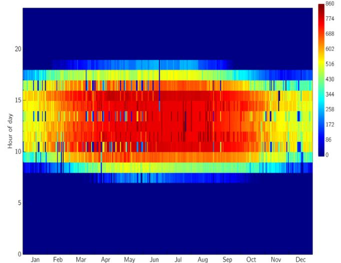
Fig.2: Hourly DNI-Cosine Product Irradiance for Parabolic Trough Collector at Sebha city [19].
