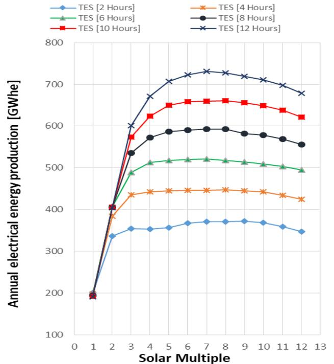
Fig.6: Variation of solar multiple and hours of storage with annual energy production for PTC plant in Sebha.
