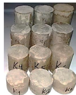
Figure 5.3 Casted Concrete Samples Ready for Gamma Ray Attenuation and Compression Tests
