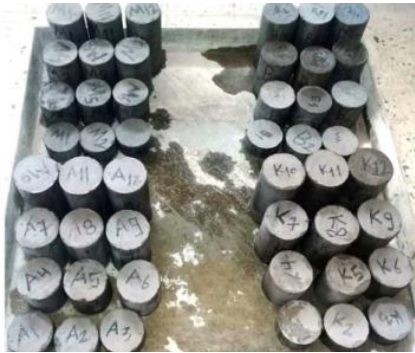
Figure 7.2. Concrete Samples Prepared for the Compression
