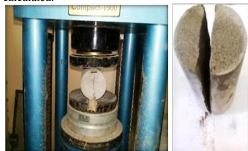
Figure 7.1 Concrete Sample under Failure of Compression Load
