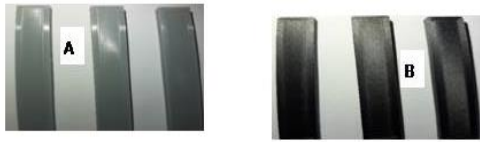
Fig 7: Shows the surface roughness of (A) PETG and (B) PETG/Carbon fiber specimens.
