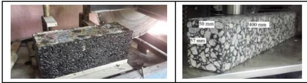
a) Block Samples Were Trimmed b) Specimens Geometry
