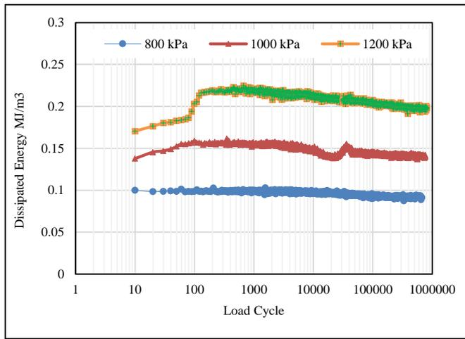
Fig 1: Impact of Stress Level on Dissipated Energy of GGCP
