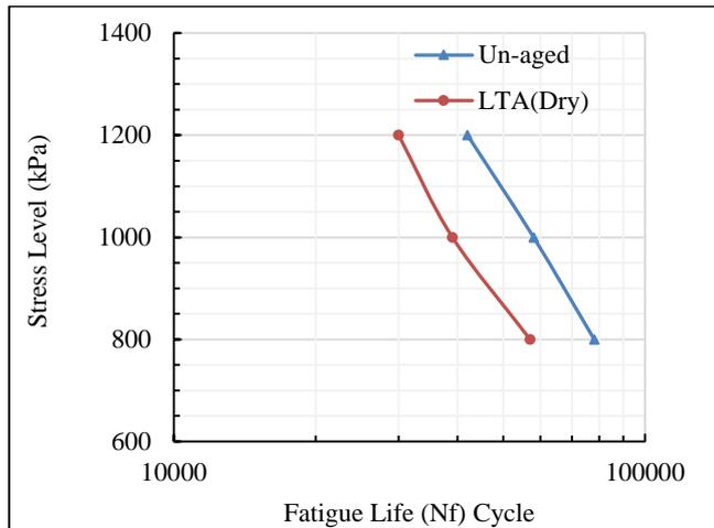
**Fig 3:** The Relationship Between Stress Level and Fatigue Life for GGCP
