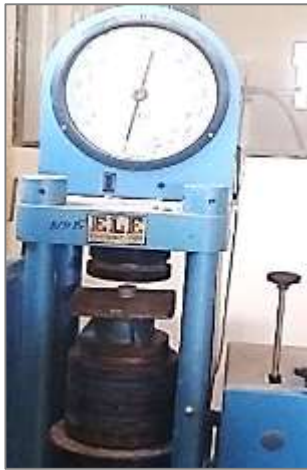
Figure 3.2. Compression Test Machine Used in the Present Work.
