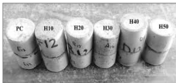
Figure 3.1. Experimental Specimen before Compression Test
