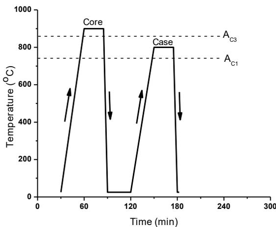
**Fig. 8:** Schematic illustration of double quenching process
