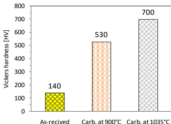
**Fig. 3:** Vickers hardness of the studied specimens before and after carburizing at 900°C and 1035°C
