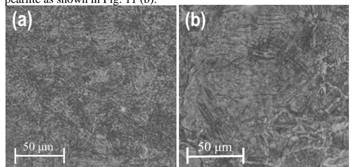
**Fig. 11:** Optical micrograph at 200x magnification: (a) case and (b) core of the carburized specimens after double quenching process
