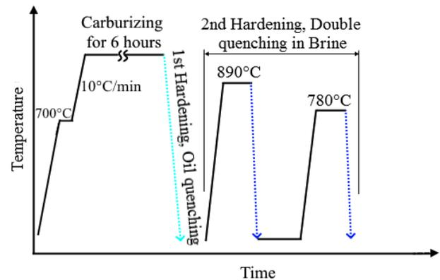
**Fig. 1:** Schematic illustration of the carburizing and hardening process
