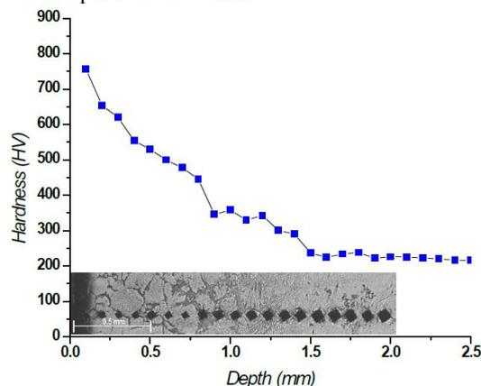
**Fig. 6:** Cross-section microhardness profiles and optical micrograph at 50x (inset) of the carburized specimen at 1035°C after direct quenching in oil
