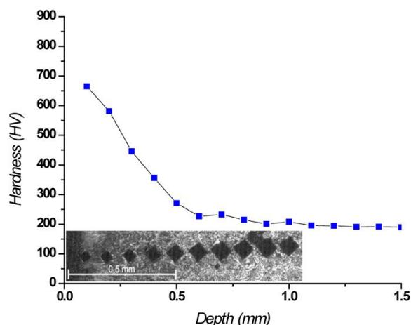
**Fig. 4:** Cross-section microhardness profiles and optical micrograph at 50x (inset) of the carburized specimen at 900°C after direct quenching in oil
