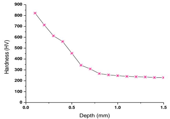
**Fig. 9:** Cross-section microhardness profiles of the carburized specimen at 900°C after double quenching in brine
