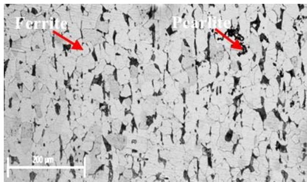
**Fig. 2:** Optical micrograph showing the ferrite and pearlite microstructure of as-received low-carbon steel (0.14 %C) before carburizing, Mag. 100x
