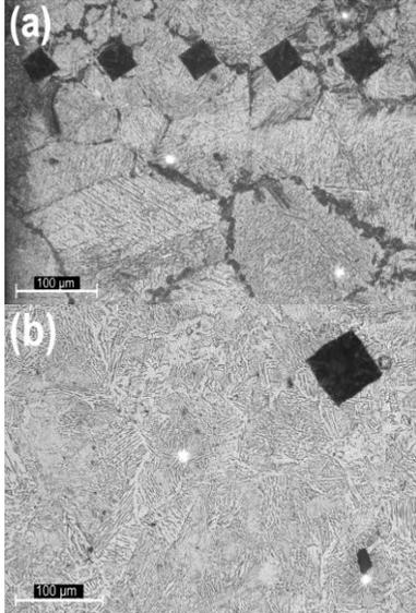
**Fig. 7:** Optical micrograph at 200x magnification: (a) case and (b) core of the carburized specimen at 1035°C after direct quenching in oil.
