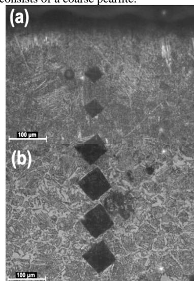
**Fig. 5:** Optical micrograph at 200x magnification: (a) case and (b) core of the carburized specimen at 900°C after direct quenching in oil
