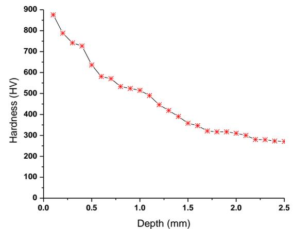
**Fig. 10:** Cross-section microhardness profiles of the carburized specimen at 1035°C after double quenching in brine
