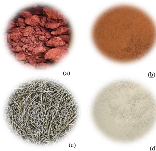
Fig. 1: Materials used (a) soil as collected, (b) sieved soil, (c) Athel leaves as collected and (d) grained Athel leaves
