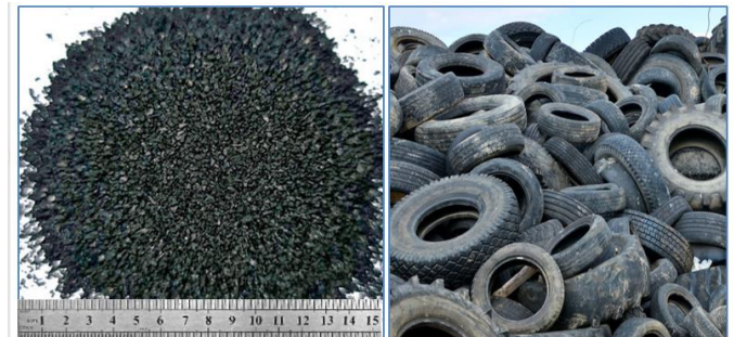
Fig. 1: Recycled rubber used in the concrete
