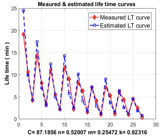
Fig. 9: The estimated Tool Life versus measured Tool Life
