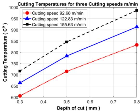
Fig. 11: The approximated temperature rises at tool chip interface based on the Nathan Cook model from eqn. 3.
