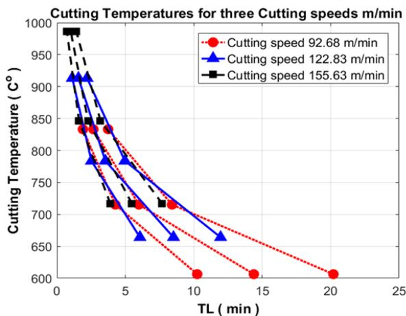
Fig. 12: The approximated temperature rises at tool chip interface versus the Tool life from eqn. 4.
