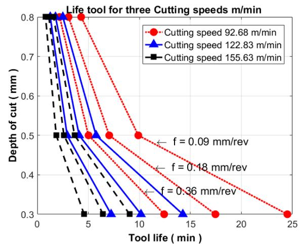
Fig. 10: The effects of cutting parameters on the tool life eqn. 8.
