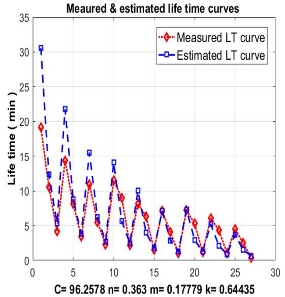
**Fig. 4:** Measured versus Estimated Tool life
