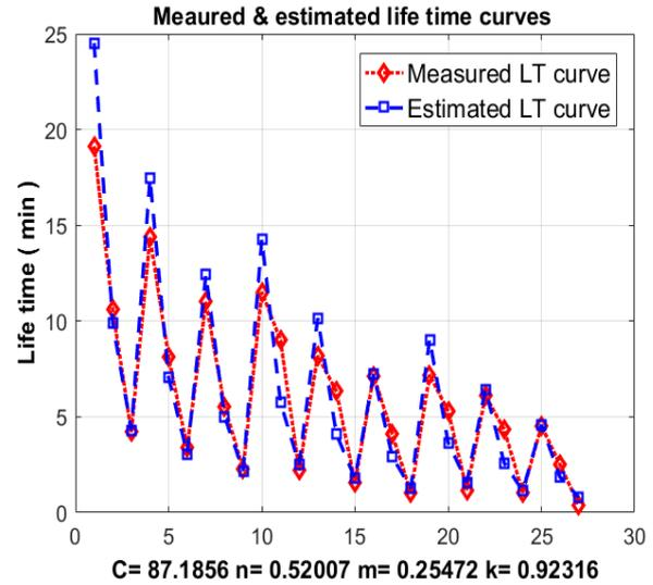
**Fig. 5:** Measured versus Estimated Tool life
