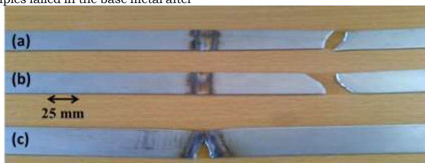
Figure 3.1 failed welded joint tested in this work
