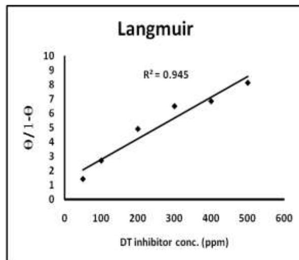
**Figureure 3.** Langmuir adsorption isotherm plot of TD at 30 °C
