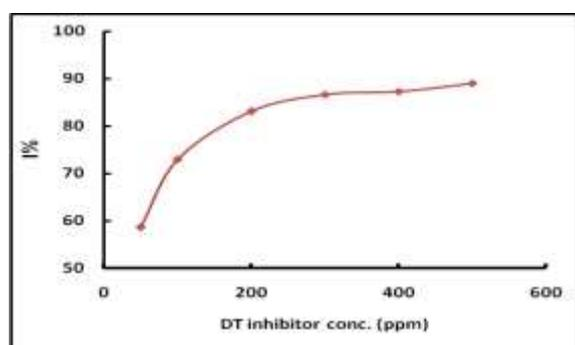
**Figure2.** The inhibition efficiency of TD at 30 °C. From the values obtained, it is obvious that there is a decrease in the corrosion rate of mild steel in the presence of (TD) when compared to the blank.
