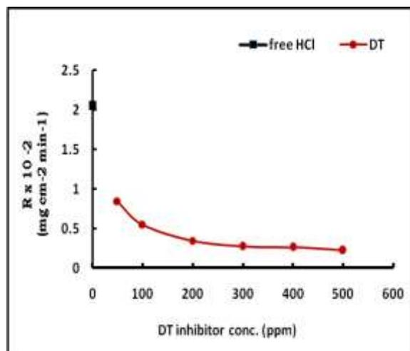
**Figure1.** Effect of the change of the TD concentration on the inhibition of mild steel in 0.5M HCl at 30°C.
