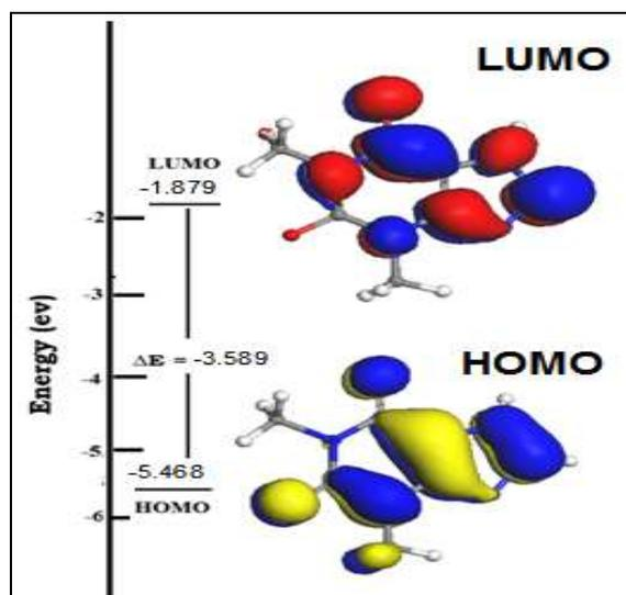
**Figure 6.** HOMO and LUMO of the neutral inhibitor molecule by DFT
