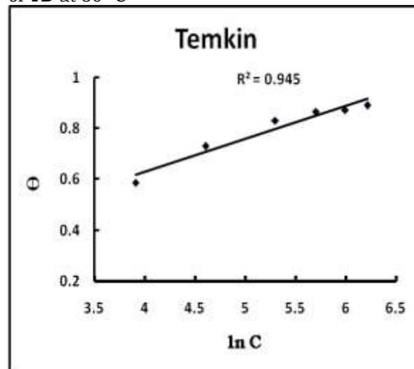
**Figureure 4.** Temkin adsorption isotherm plot of (TD) at 30 °C
