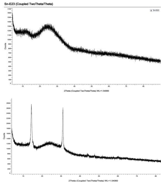
**Figure (6):** X-ray diffraction patterns of 150nm as deposited and annealed (350 °C) SnSe4 thin films
