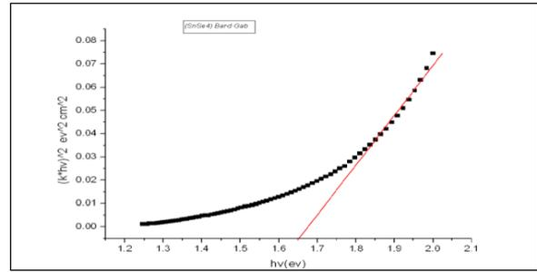
**Figure (5):** Shows relation between  $(k * hv)^{\frac{1}{2}}$  and photon energy of as deposited 160 nm SnSe4.
