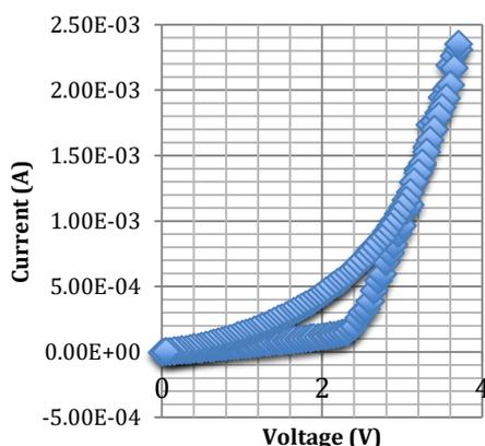
**Figure (9):** Change from crystalline to amorphous after applying pulse 1.6v at 20 Microsecond
