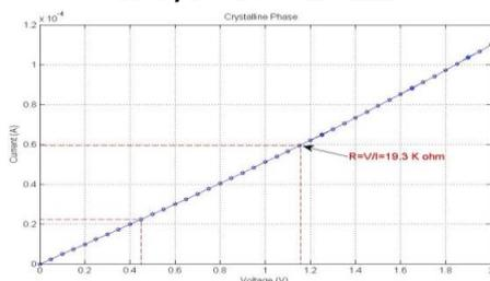
**Figure (8):** Shows the value of resistance during crystalline phase
