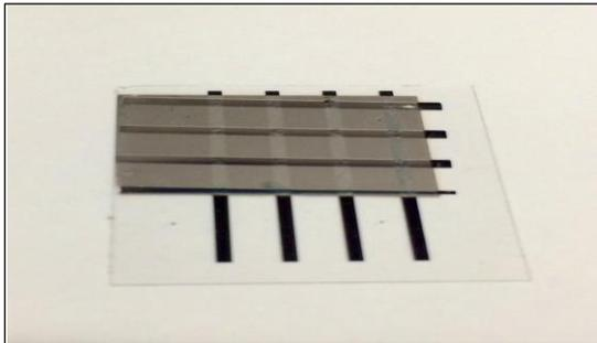
**Figure (3):** Final shape of PCM with 150 SnSe4 thin film
