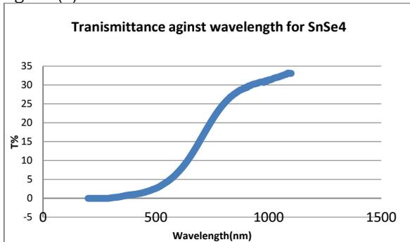
**Figure (4):** Illustrates transmittance with wavelength for 160 nm SnSe4 thin films alloys
