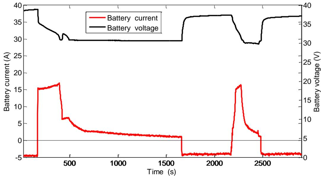
**Fig. 5:** Battery voltage and current during different flight phases, scenario with low SoC
