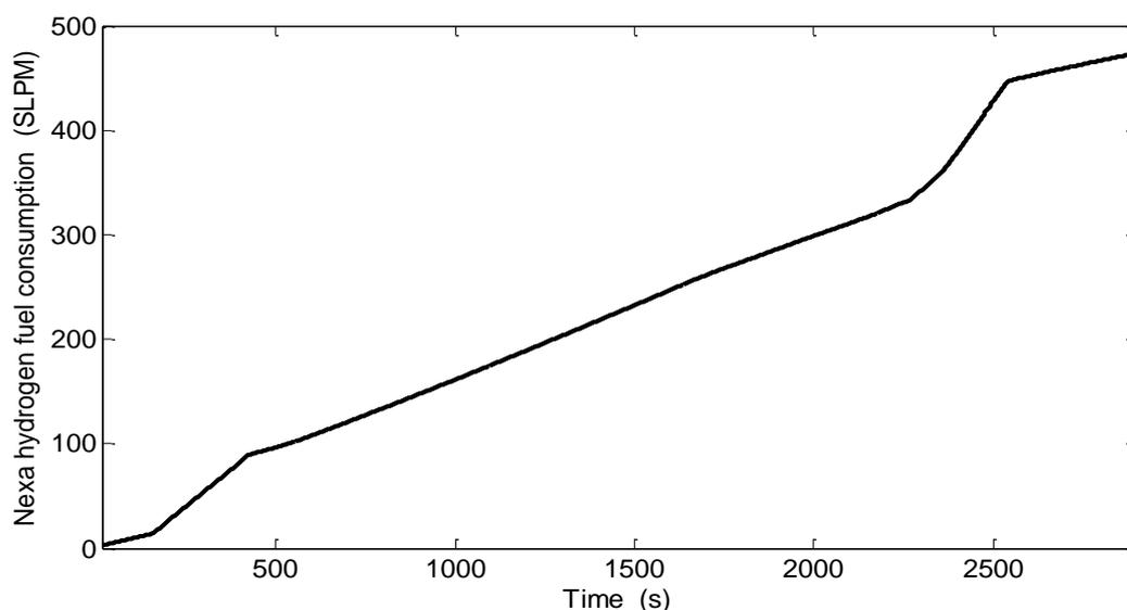
**Fig. 6:** Nexa fuel consumption during different flight phases, scenario with low SoC
