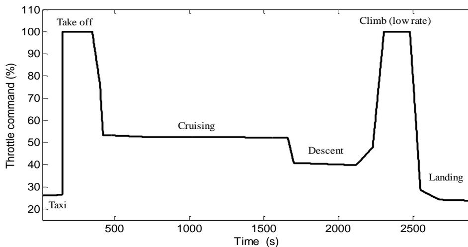
**Fig. 3:** Throttle commands during different flight phases
