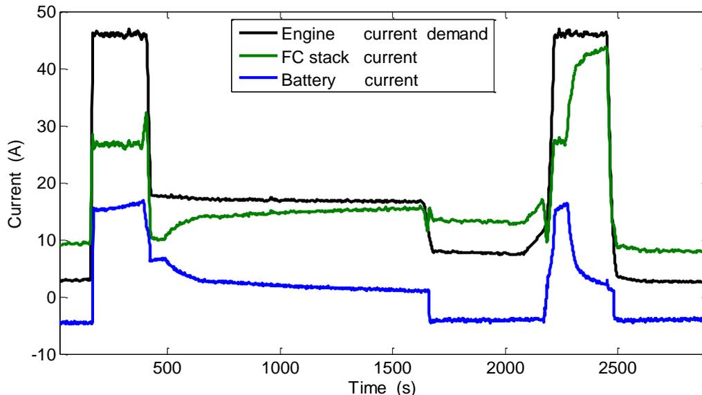
**Fig. 4:** Engine current demand, FC current and battery current during different flight phases
