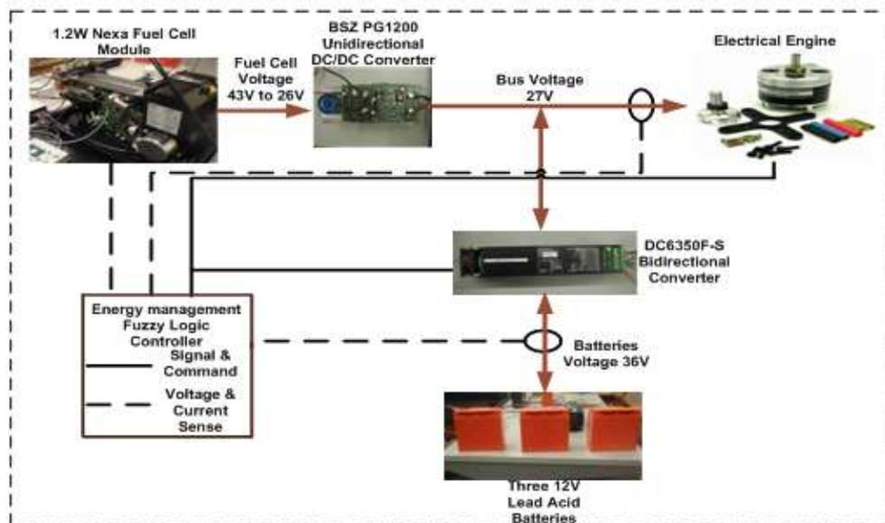
**Fig. 2:** Fuel cell/battery hybrid propulsion system
