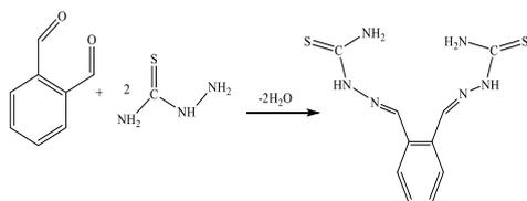
**Scheme -2:** Synthesis of Schiff base (H<sub>2</sub>L)
