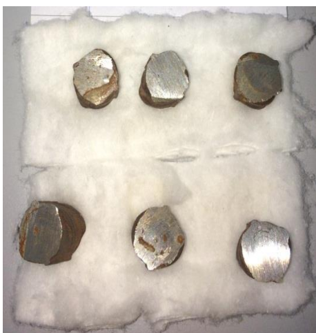
Figure 2 - 14 mm Ø Steel Specimens
