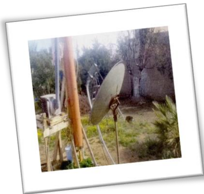
Fig. (3-a,3-b): solar desalination unit with a evaporation and condensation cycle
