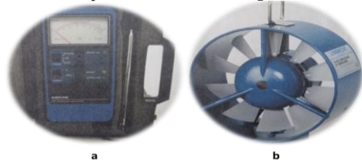
Fig. 6: digital air flowmeter (a), speedometer (b)
