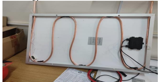
Figure 5 Description of the cooled photovoltaic.
