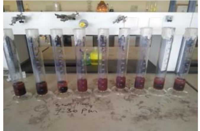
Figure (11) Graduated Tester That By gum Arabic solution in (Gaberoun Water Leak & distilled) water.
