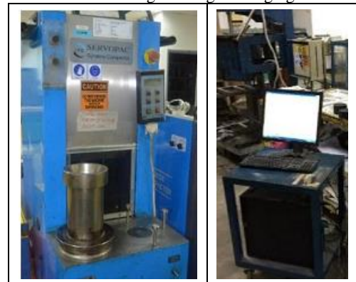
Fig. 2: Servopac gyratory compactor
