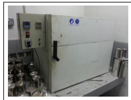
Fig. 3: Oven Draft Used for Simulating the Long-Term Aging Process
