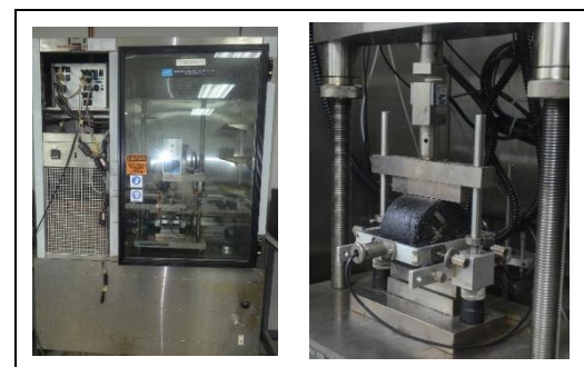
Fig. 6: UTM-25 Set Equipped with an Environmental Chamber for MR Test
