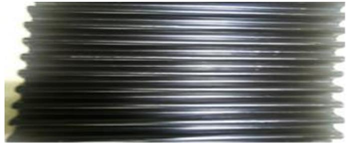
Fig. 5: corrugated plate fabricated and coated
