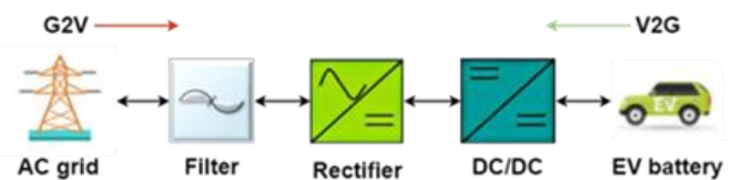
Fig. 1: Bidirectional energy flow of V2G
