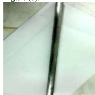
Figure. (3) The general corrosion on the test sample after immersion of 95 days in natural seawater environment and after removing all existing corrosion product and well surface cleaning.
